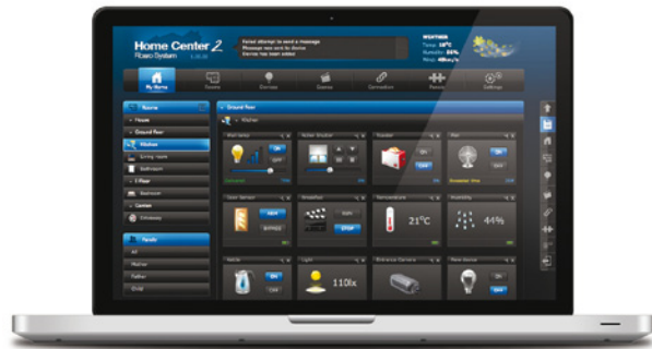
Configuration interface FIBARO HC2
